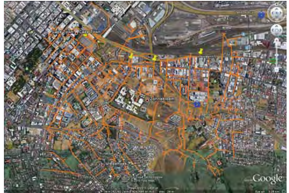
FIGURE 4.34: EXISTING SEWER SERVICES
